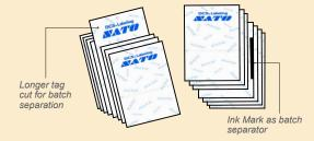
The printer separates tags by cutting the first tag longer or using the ink roller mechanism to place an ink mark on the side of each batch separator tag.
